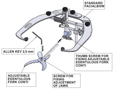
**Image 2:** Elite Edentulous Fork being mounted on the Elite Facial Arch: the fork is fixed by tightening the arch fixing screw.
