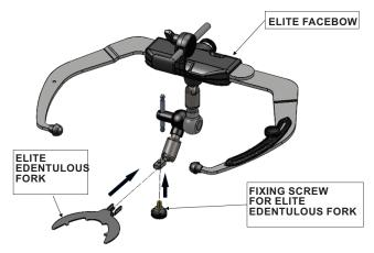
**Image 3:** Dentate Fork being mounted on the Standard Face Bow: the fork is fixed by tightening the bow clamping throttle.
