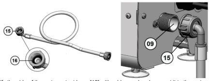
•Identify the side of the water output hose [18] with rubber end and connect it to the water outlet [14] of the Plaster Cutter, located in the upper part. The other end shall be placed at the location, where the water will be disposed. The water disposal location shall be tilted in relation to the water outlet of the Plaster Cutter, in order to facilitate the water flow, avoiding clogging.
